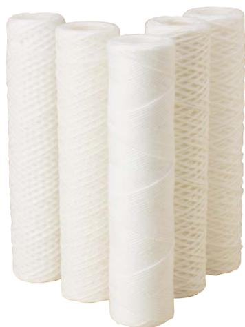
**Pentair Pentek CW Series Cartridges** are manufactured from a durable polypropylene cord that is wound around a rigid polypropylene core. They are an economical solution to reduce fine sediment, including sand, silt, rust and scale particles.
