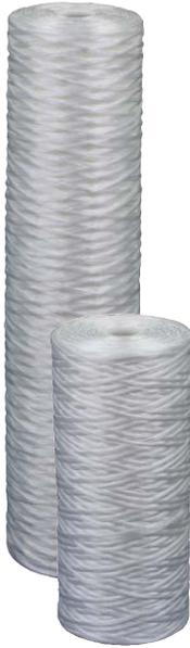
**Pentair Pentek WPX-BB Series Cartridges are manufactured in 10" and 20" lengths and in 4.5" diameters from a durable polypropylene string that is wound around a rigid polypropylene core. The WPX-BB Cartridges are an economical solution to reduce fine sediment including rust, sand and scale particles.**
