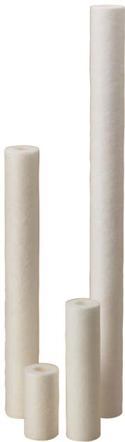
The Pentair Pentek P Series Cartridges are manufactured from pure 100% polypropylene fibers. The fibers have been carefully spun together to form a true gradient density from outer to inner surfaces.
