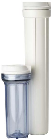
**Pentair Pentek Standard Flat Cap Filter Housings are manufactured of a durable polypropylene or clear Styrene-Acrylonitrile (SAN). All are equipped with 3/4" NPT inlet and outlet ports. These housings are available in both 10" and 20" lengths and will accommodate a wide range of 2-1/2" to 2-7/8" diameter cartridges. The reinforced polypropylene cap offers an optional pressure-relief button on the inlet side to relieve pressure inside the housing when changing filter cartridges.**
