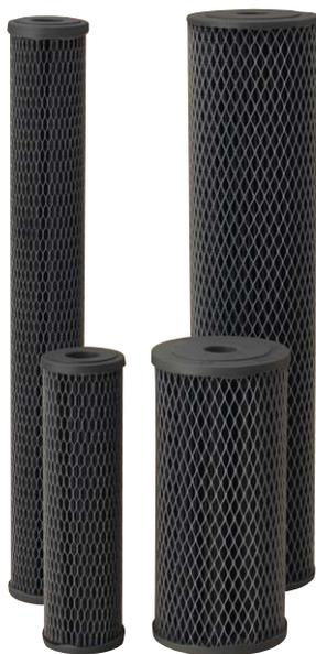
**Pentair Pentek NCP Series Cartridges are constructed from a carbon-impregnated non-cellulose media. They offer sediment filtration, as well as taste, odor and chlorine taste & odor reduction in one cartridge. Unlike cellulose cartridges, NCP Series Cartridges can be used for municipal and non-chlorinated water applications.**
