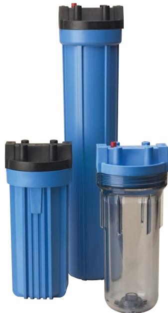
**Pentair Pentek Standard Filter Housings are manufactured of a durable polypropylene or clear Styrene-Acrylonitrile (SAN). All are equipped with 3/4" NPT inlet and outlet ports. Standard Filter Housings are available in both 10" and 20" lengths and will accommodate a wide range of 2-1/2" to 2-7/8" diameter cartridges. The reinforced polypropylene cap offers an optional pressure-relief button on the inlet side to relieve pressure inside the housing when changing filter cartridges.**
