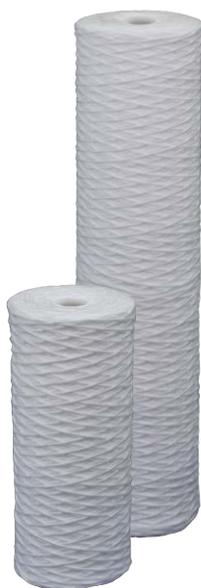
**Pentair Pentek WP-BB Series Cartridges are manufactured in 10" and 20" lengths and in 4.5" diameters from a durable polypropylene string that is wound around a rigid polypropylene core. The WP-BB Cartridges are an economical solution to reduce fine sediment including rust, sand and scale particles.**
