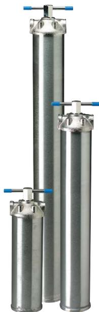
**Pentair Pentek ST Series Stainless Steel Filter Housings effectively provide heavy duty filtration for smaller filtration systems and point-of-use applications. Supplying flow rates of up to 20 gpm (76 Lpm), at a maximum water temperature of 300°F (149°C), ST Series Housings are ideal for hot water and high-pressure applications not suited for plastic housings.**
