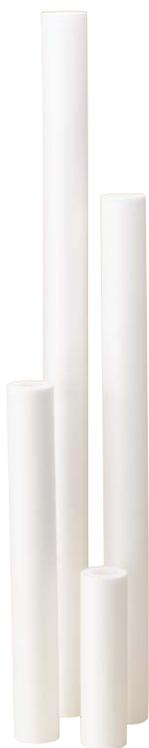
**Pentair Pentek Polydepth<sup>®</sup> Filtration Cartridges are constructed of thermally bonded polypropylene microfibers to ensure high efficiency. The filter incorporates a rigid polypropylene center core for increased collapse strength and durability. This thermal bonded micro-fiber construction has minimal fiber release, consistent flow rate and superior filtration performance. It also is not brittle or prone to breakage problems like resin-bonded cartridges.**
