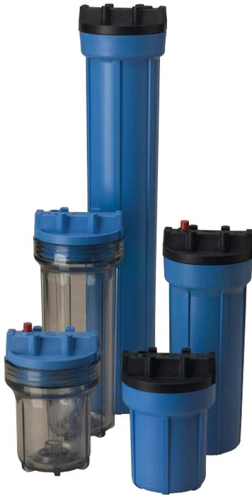
**Pentair Pentek<sup>®</sup> Slim Line<sup>®</sup> Filter Housings** are available in either reinforced polypropylene or clear Styrene-Acrylonitrile (SAN) in 5", 10" and 20" lengths. The black or blue reinforced polypropylene housing caps are available with 1/4", 3/8" or 1/2" NPT connections. Four bosses are molded into every cap for mounting purposes.
