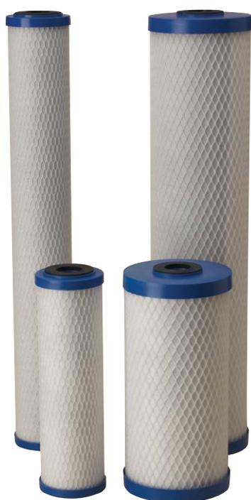
The Pentair Pentek EP Series Carbon Block Cartridges are manufactured using a process that yields a cartridge with a nominal 5-micron filtration rating and high dirt-holding capacity. A high porosity design helps prevent the cartridge from plugging before its adsorption capacity is exhausted, maximizing the utilization of the carbon while maintaining low pressure drop.
