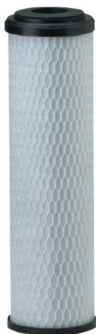
**The Pentair Pentek C8 Series Cartridge offers an economical solution for general purpose water filtration needs. Constructed of a carbon impregnated cellulose media, this dual-purpose cartridge filters chlorine taste & odor, bad taste & odor and sediment particles\*. The cartridge has a high dirt-holding capacity and can be used in a wide variety of applications.**
