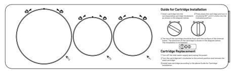
Twist anti-clockwise to remove, clockwise to install
