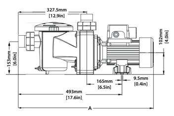
A: 0.25KW = 585mm 0.75KW = 607mm 0.375KW = 585mm 1.10KW = 642mm
