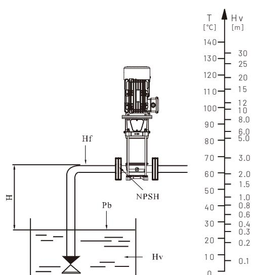
Check to ensure that the pump will not be in cavitation .
