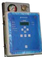
CS 400 Commercial Backwash Controller This controller is programmable and controls every aspect of the backwash cycle once initiated. Backwash can be initiated three ways: by an operator with the touch of a button, by a signal from a master controller (such as the AK600), or by a signal from an optional differential pressure switch (CS400-DP). Stored backwash data and history, alarms, and calculated backwash cycle times are also features of the CS400 controller, as are relays for communication with the heater, pump and Acu Drive.
