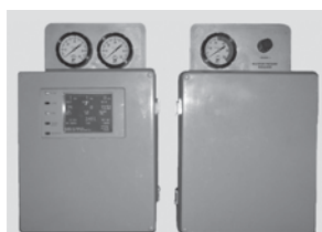
CA 100 Fully Automatic Backwash Controller This is the most comprehensive backwash controller and can be readily reprogrammed to initiate backwash automatically based on differential pressure (integral pressure transducers are standard), time (internal seven-day clock with battery back-up is standard), flow (with optional flow sensor), or any combination of the above. The controller has real-time display of operation mode, filter flow rate, and water temperature (with optional temperature probe). Also, includes Energy Saver Mode for simple On/Off pump scheduling and various interlocks and relays to communicate with other equipment (pump, heater, Acu Drive).
